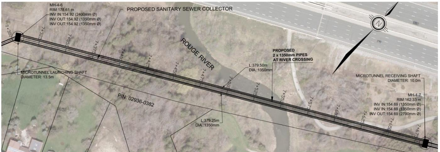
Figure 7-10 Conceptual Alignment at Rouge River Crossing
