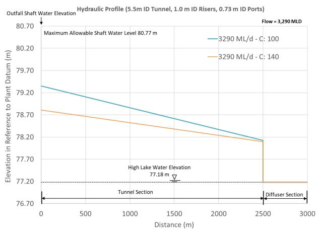
Figure 10.14 Outfall Hydraulic Profile under C-100 and C-140 Hazen-William Friction Factors
