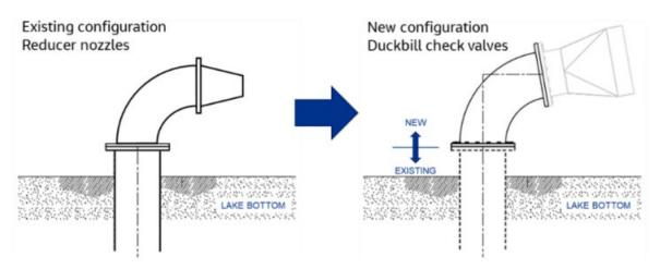
Figure 10.3 Existing and New Diffuser Port Configuration
