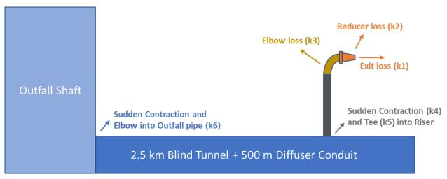
Figure 10.13 Minor Loss K Factors for Outfall Tunnel, Risers, and Diffuser
