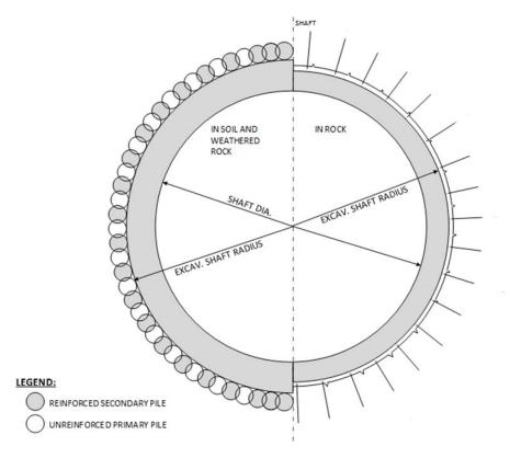
Figure 10.17 Shaft Excavation Support Types
