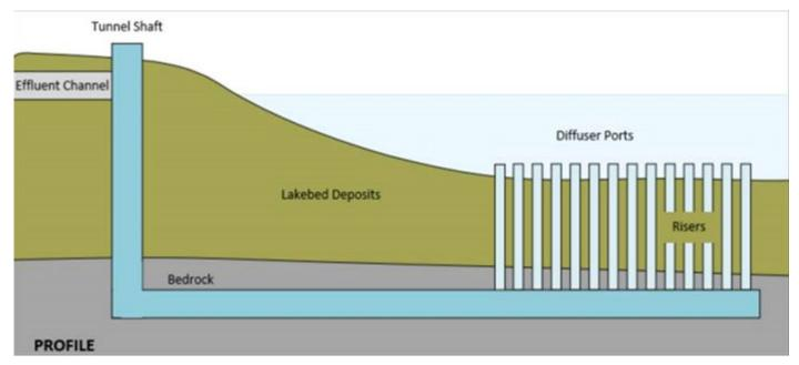
Figure 10.18 Conceptual Profile of Outfall Tunnel
