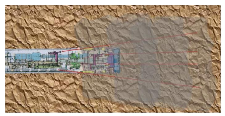
Figure 10.20 Grouting from within the TBM
