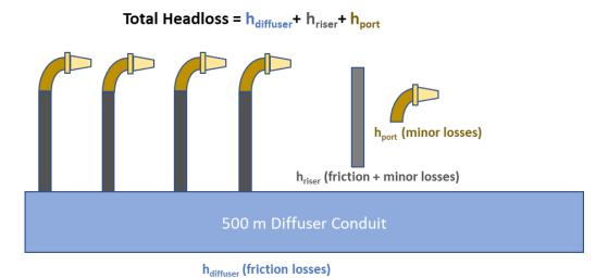
Figure 10.12 Illustration of Headloss Components for the Diffuser Section of the Outfall
