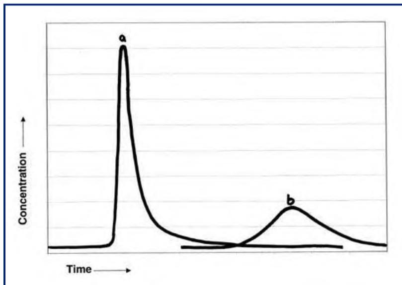
**Figure 25. Example Graph of Rhodamine WT Concentration Versus Time for a Slug Injection Test.**
