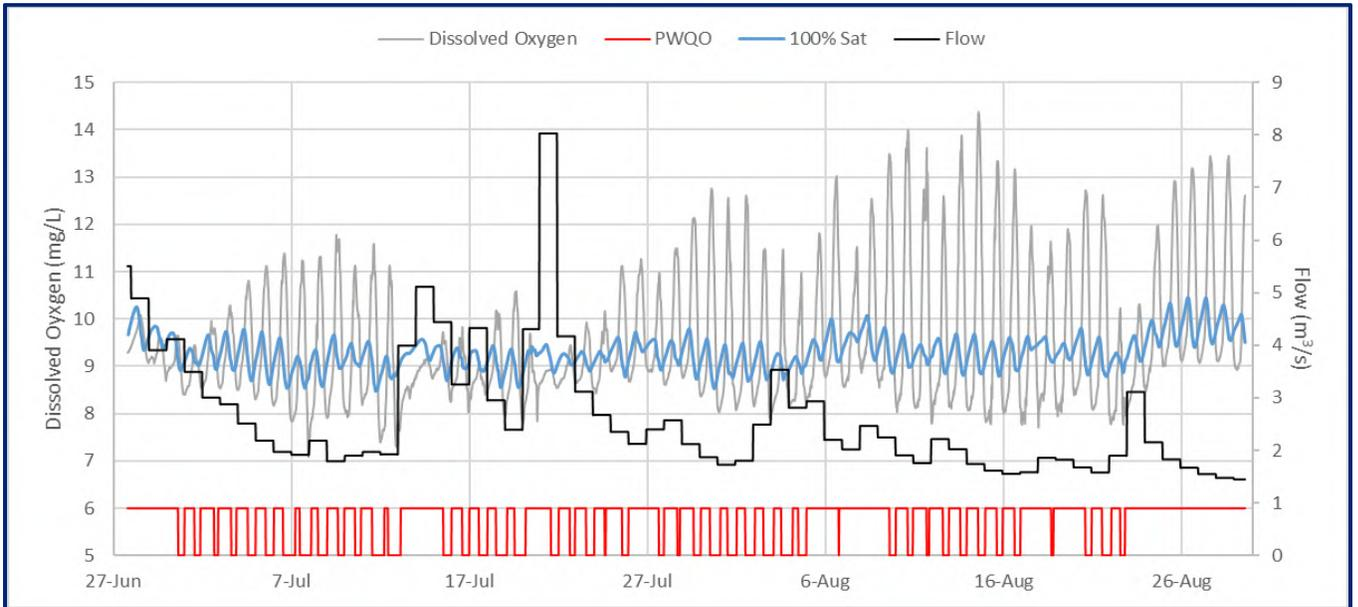
**Figure 13. Continuous Dissolved Oxygen and Temperature Measurements in the Humber River 350 m Downstream of the Nobleton WRRF discharge.**
