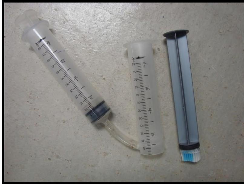
**Figure 38. Application of Syringe Periphyton Sampler in the Field.**
