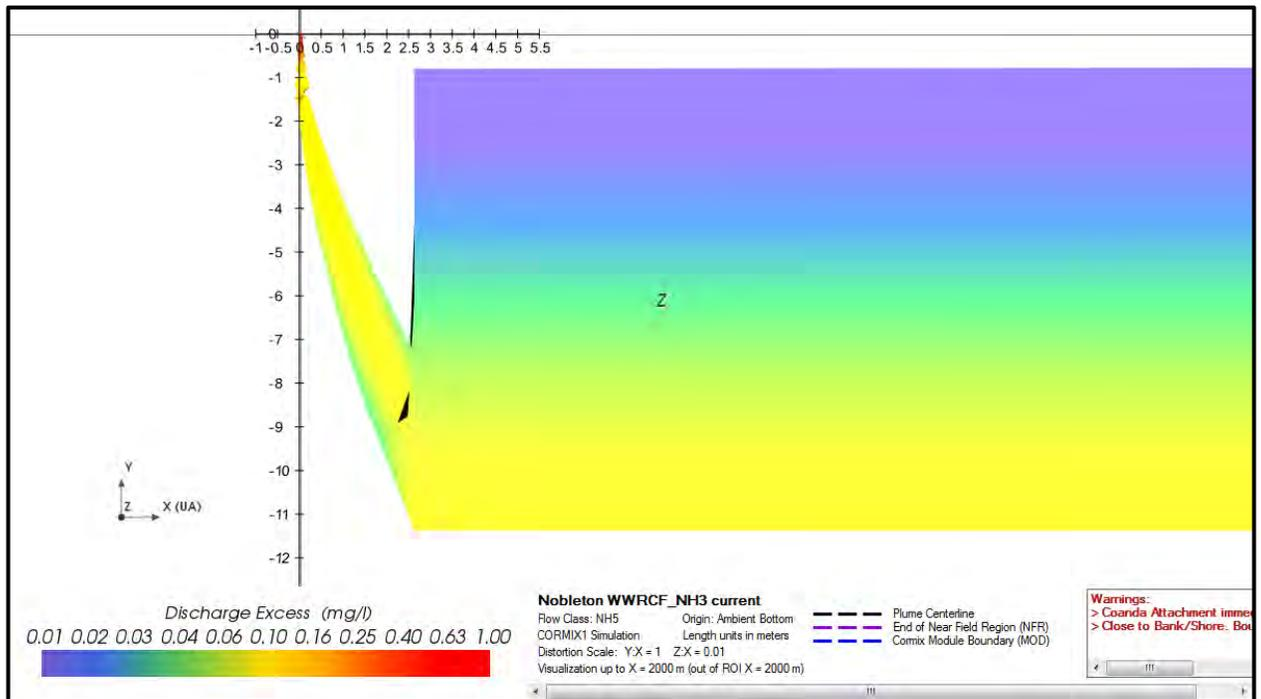
**Figure 5 Plan view of model prediction for Nobleton WRRF Effluent Discharge**
