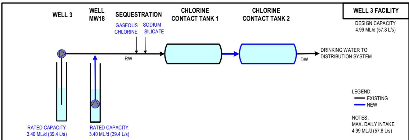
Figure 4-6. Alternative A7b Schematic Diagram
