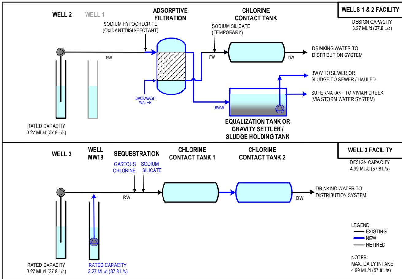
Figure 4-7. Alternative A7c Schematic Diagram
