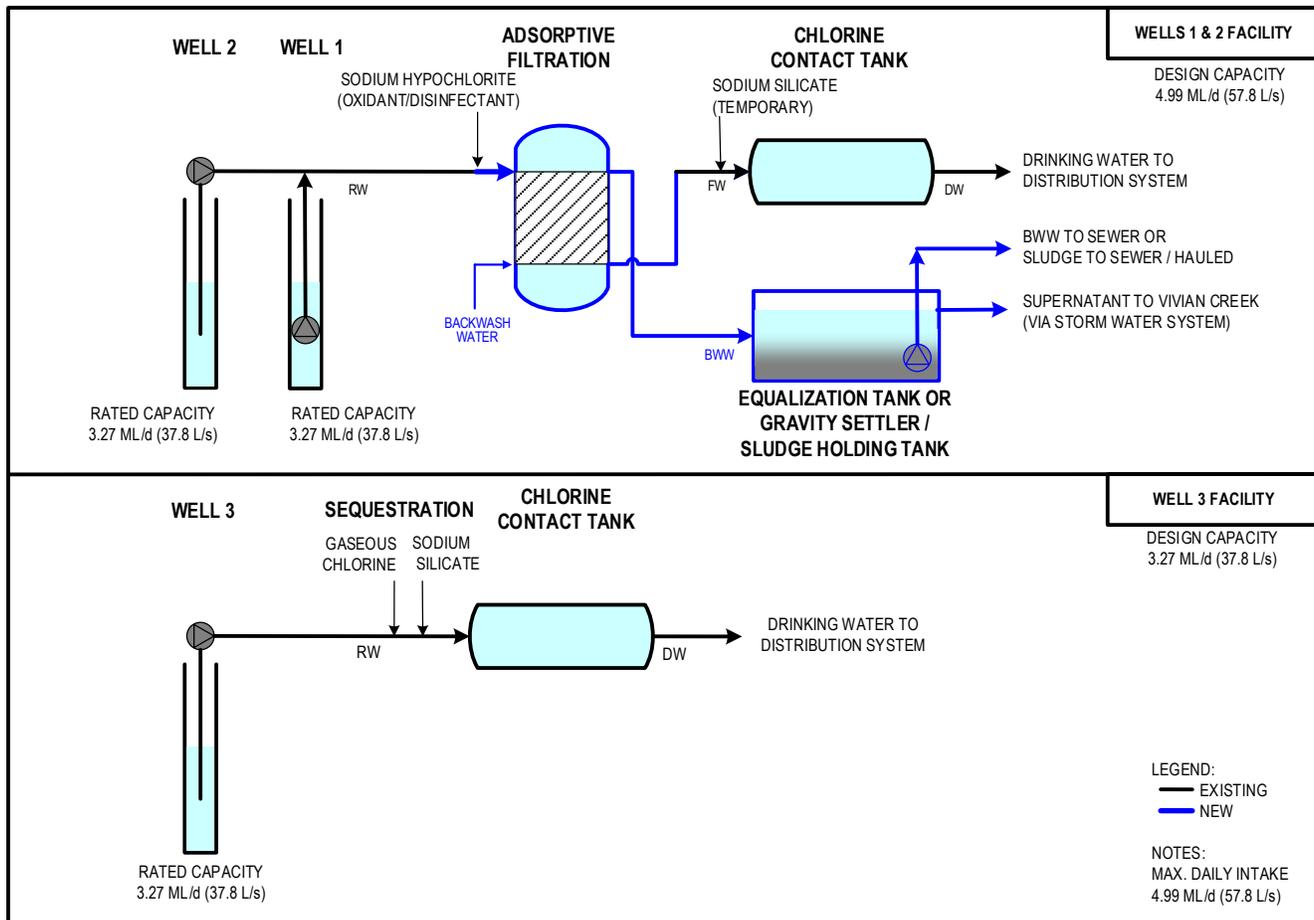
Figure 4-4. Alternative A6 Schematic Diagram
