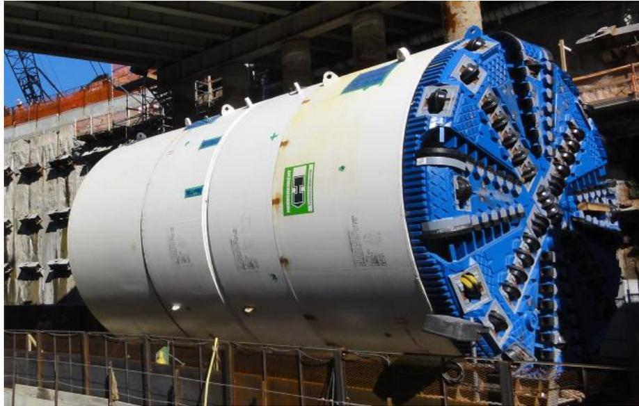
**Pressurized Face Tunnel Boring Machine**
