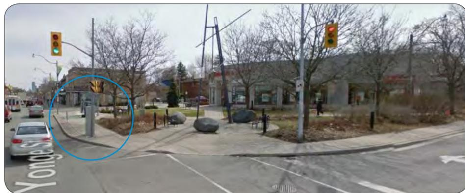
The image below shows a traffic control cabinet interrupting the flow of a new urban plaza. This traffic control cabinet was most likely originally located within the site triangle and did not get moved when the adjacent property was urbanized and the plaza was developed. The transformer box also negatively impacts the overall design of the new plaza.
