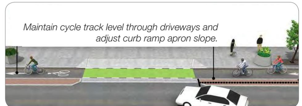
Maintain cycle track level through driveways and adjust curb ramp apron slope.
