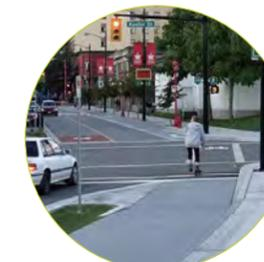
Precedent image of a raised two-way cycle track with vertical separation from pedestrian sidewalk
