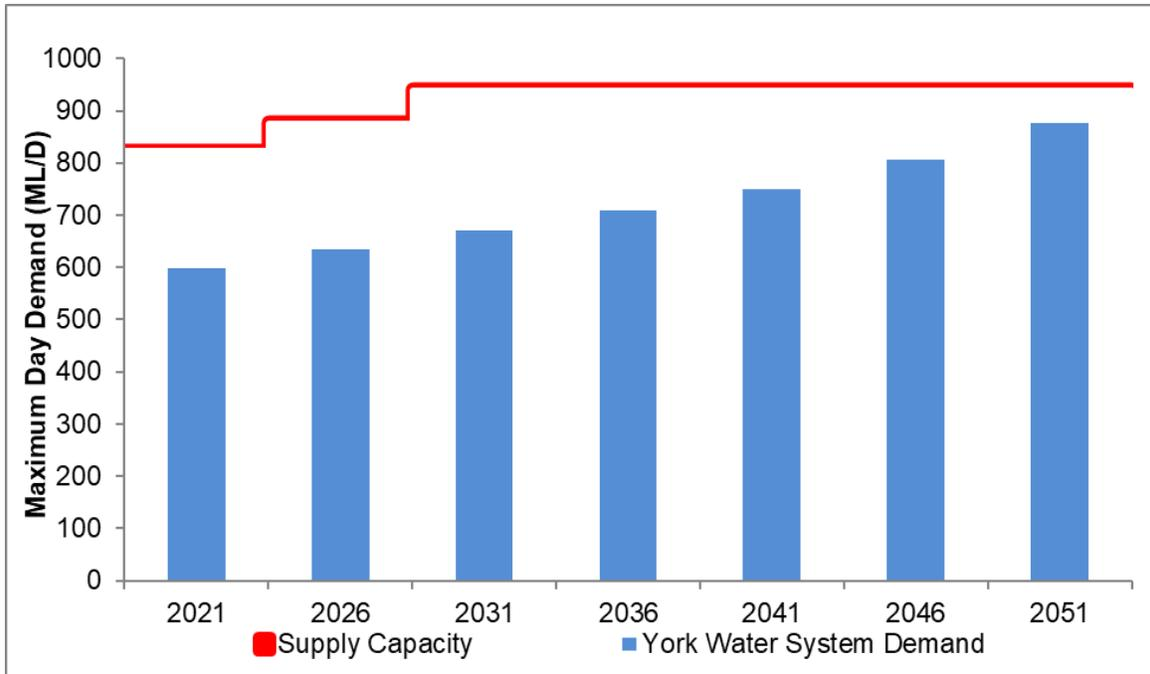
**Figure 1.4** compares the forecasted maximum day water demands to the planned supply capacity in the Georgina Water System. This figure includes the planned water transfer to support the introduction of Lake Simcoe supply into East Gwillimbury and Newmarket through the proposed Northern Connection expected to be completed in 2041. It is estimated that approximately 70% of the Georgina planned supply will be used to meet the 2051 maximum day water demand.
