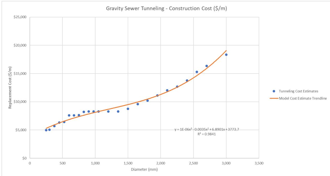
**Table 3 – Master Plan Unit Rates – Gravity Sewer Tunneling**
