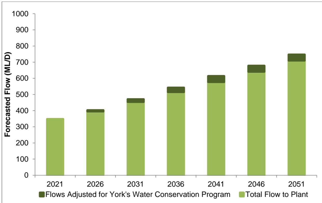
**Figure 2.2** shows the forecasted average day flows to the proposed Water Reclamation Centre compared to the planned phased capacity. The proposed Upper York Water Reclamation Centre (WRC) capacity has been planned to meet estimated increases in future wastewater flows in the service area to 2051 and beyond. This capacity is contingent on approval of the Individual Environment Assessment completed in 2014 and future Environmental Assessment(s) for planned expansion.
