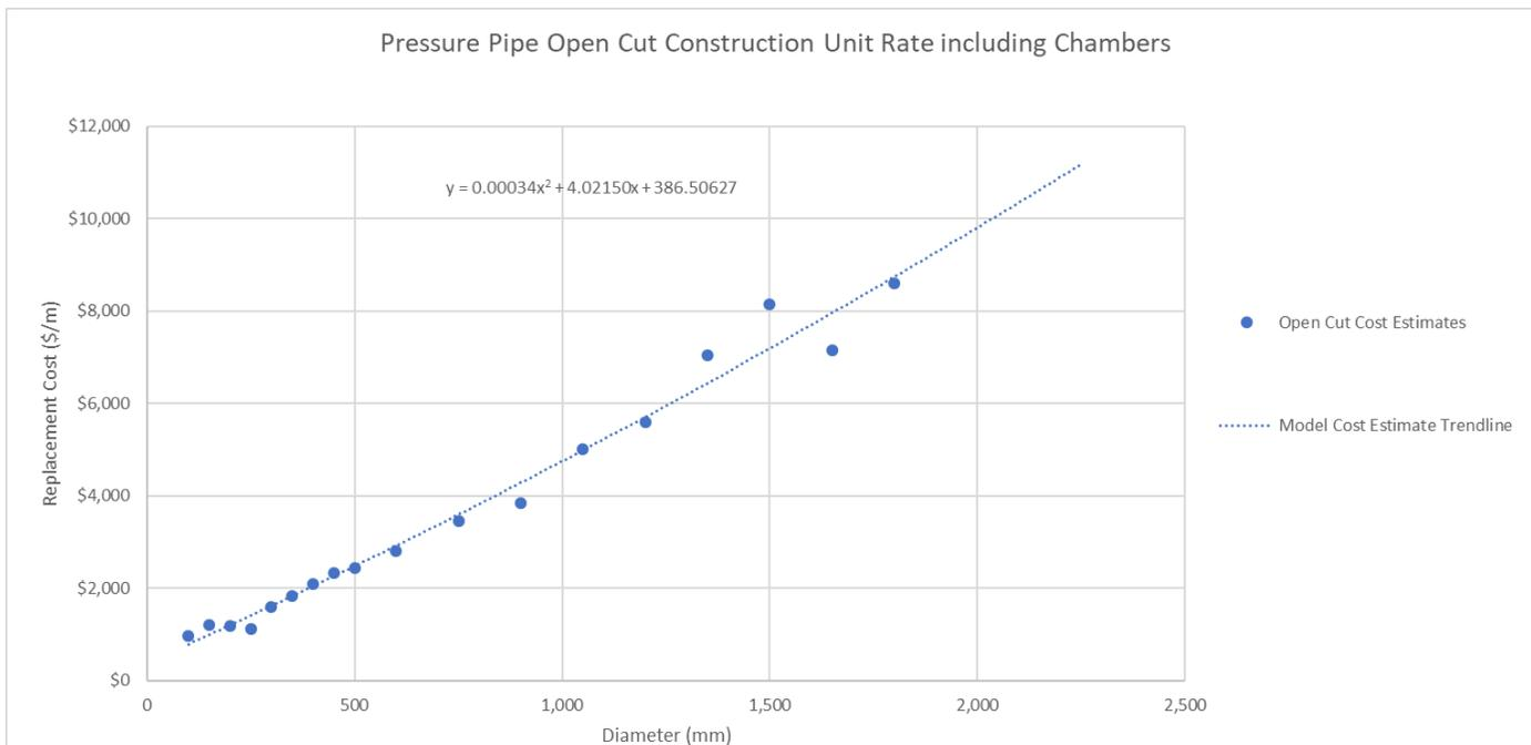
**Table 11 – Master Plan Unit Rates - Pressure Pipe – Open Cut**
