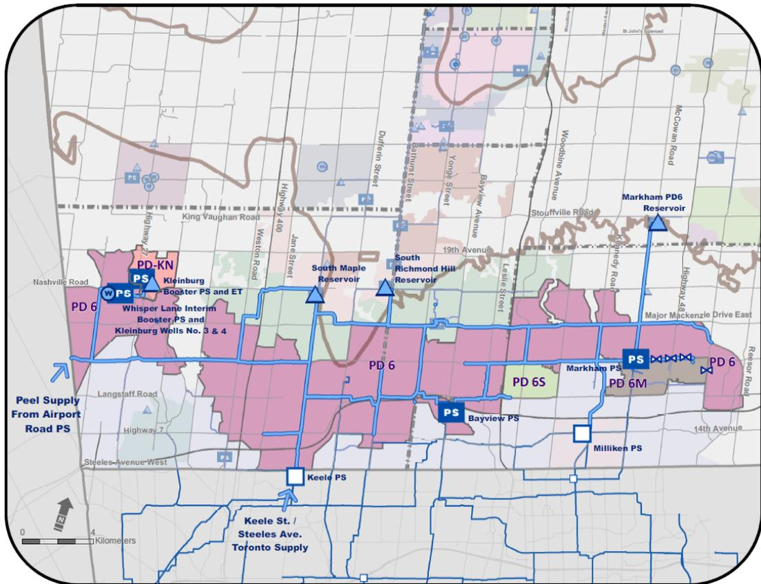
In 2010, Lake Ontario supply was introduced to the **Stouffville Water System** with the commissioning of Stouffville Zone 2 Pumping Station, which draws water from the Markham PD6 Reservoir. The existing five groundwater wells remain in place to support long term drinking water requirements. Delivery of supply in Stouffville is accomplished through three pressure zones:
