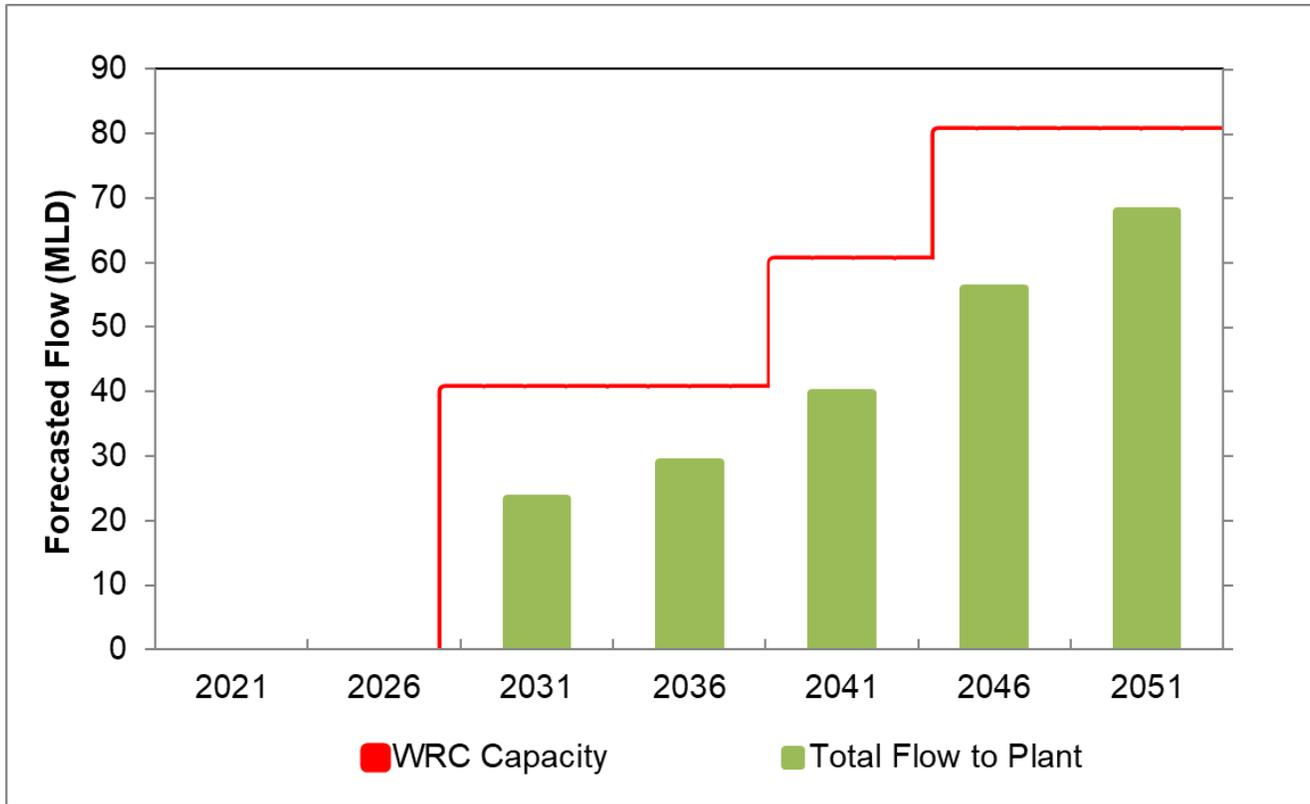
**Figure 2.3** compares the forecasted average day flow to the existing and planned capacity of Keswick Water Resource Recovery Facility (WRRF). Keswick WRRF capacity is expected to be adequate support wastewater treatment needs of the growing population in compliance requirements of the Lake Simcoe Protection Plan.
