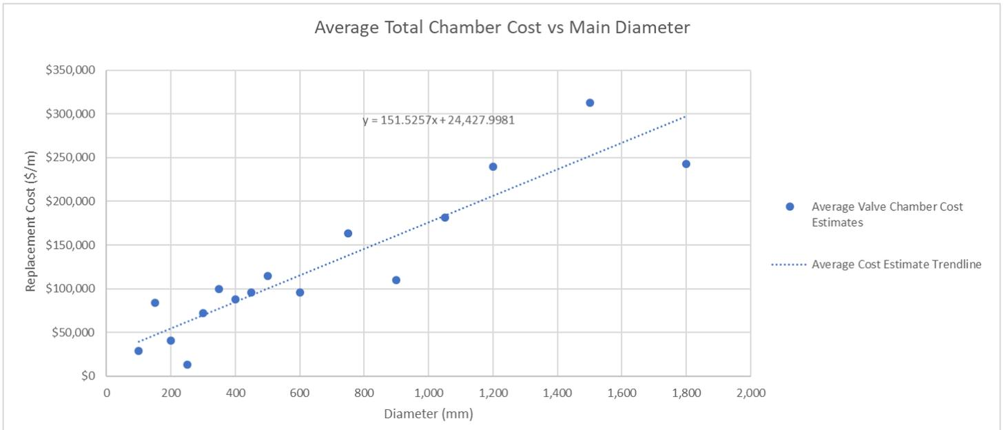
**Table 13 – Master Plan Unit Rates – Valve Chamber**
