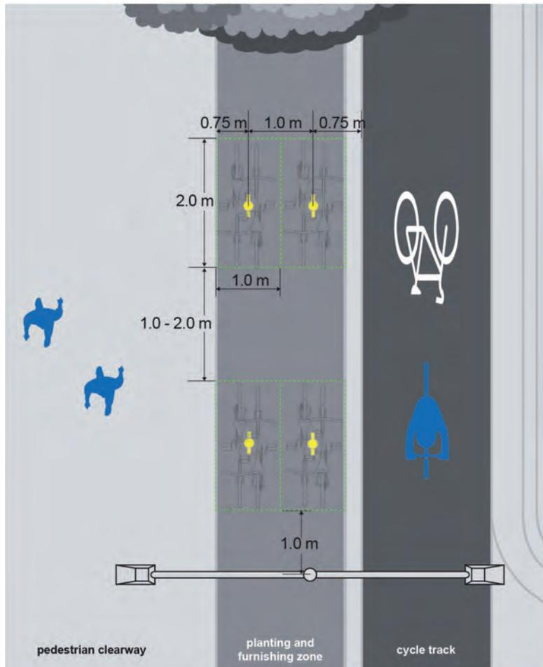
For in-boulevard parking perpendicular to the street, the centre of the bicycle rack should be:
