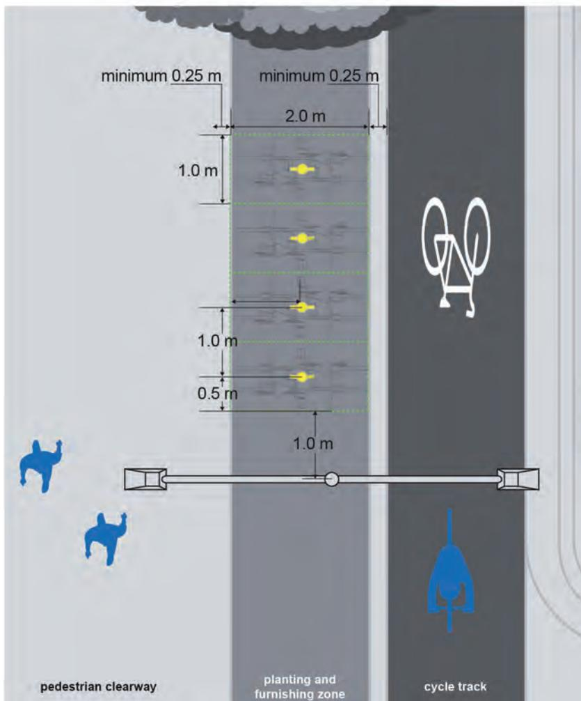
When bicycle parking is located in on-street car parking stalls, bicycle racks are typically oriented perpendicular to the street (Exhibit 9-12). The centre of the racks should be at least 1.0 m from the curb face. The first and last rack in a row should each be at least 1.0 m from the adjacent parking stall.
