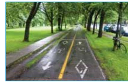
Figure 4.7 – Two-way In-Boulevard Pathway with Adjacent Sidewalk
