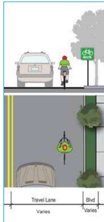
Figure 4.27 – Signed Bike Route with an Adjacent Sidewalk
