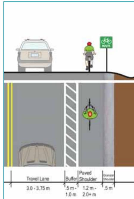
Figure 4.34 – Signed Bike Route with a Buffered Paved Shoulder
