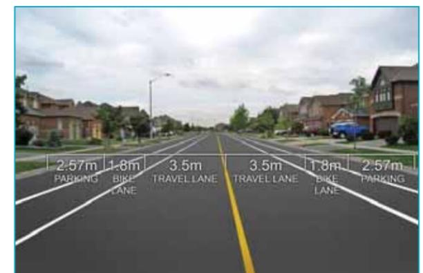
Figure 4.58 – Option 2: Bicycle Lanes with On-Street Parking and Sidewalks on Both Sides
