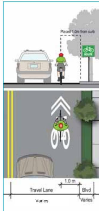
Figure 4.28 – Signed Bike Route with Optional Sharrow Adjacent to Sidewalk
