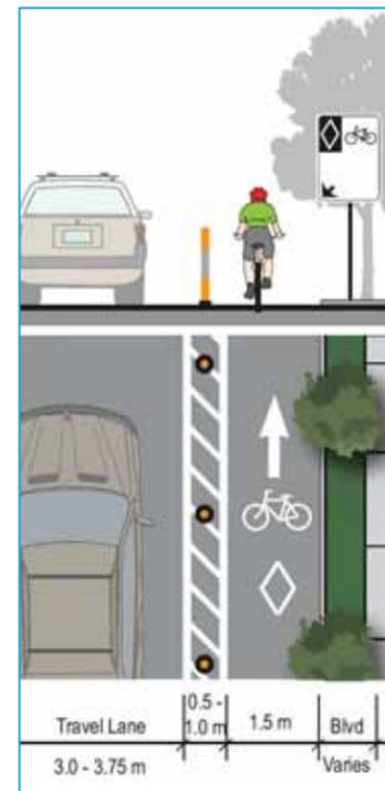
Figure 4.43 – Separated Bicycle Lane with Flex Bollards
