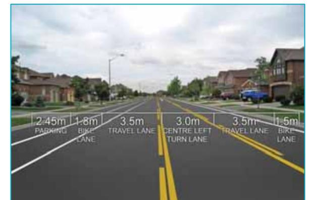
Figure 4.57 – Option 1: Bicycle Lanes with On-Street Parking on One Side, Sidewalks on Both Sides
