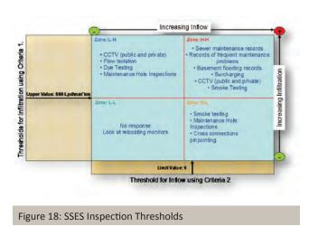
The system response is then used to determine any potential data requirements to pinpoint the sources of flows. By slightly modifying the matrix shown in Figure 18, it can be used as a guideline for selecting the appropriate inspection activities and the specific data requirements (see Figure 19 below).
