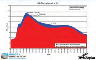
The top curve represents the expected flow at the SEC (near the community of Boxgrove in the Town of Markham) under a 25-year storm event in 2031. Simulation results predict the peak flow to be 13.3 m3/s. The lower curve represents a hypothetical event that generates a peak flow of 12.0 m3/s (10% less than 13.3 m3/s). As the analyzes reveals, the difference in volumes is approximately 71 ML over a 24-hour period.
