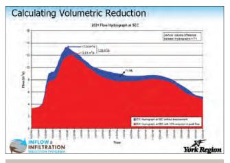
Figure 10: Calculating Volumetric Reduction
