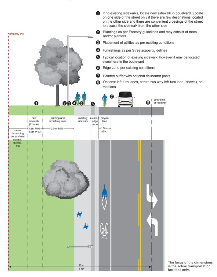
Exhibit 4-30. Retrofit (36 m ROW) - Buffered bike lanes installed as part of a road reconfiguration from four travel lanes to two travel lanes with a centre two-way left-turn lane or medians
