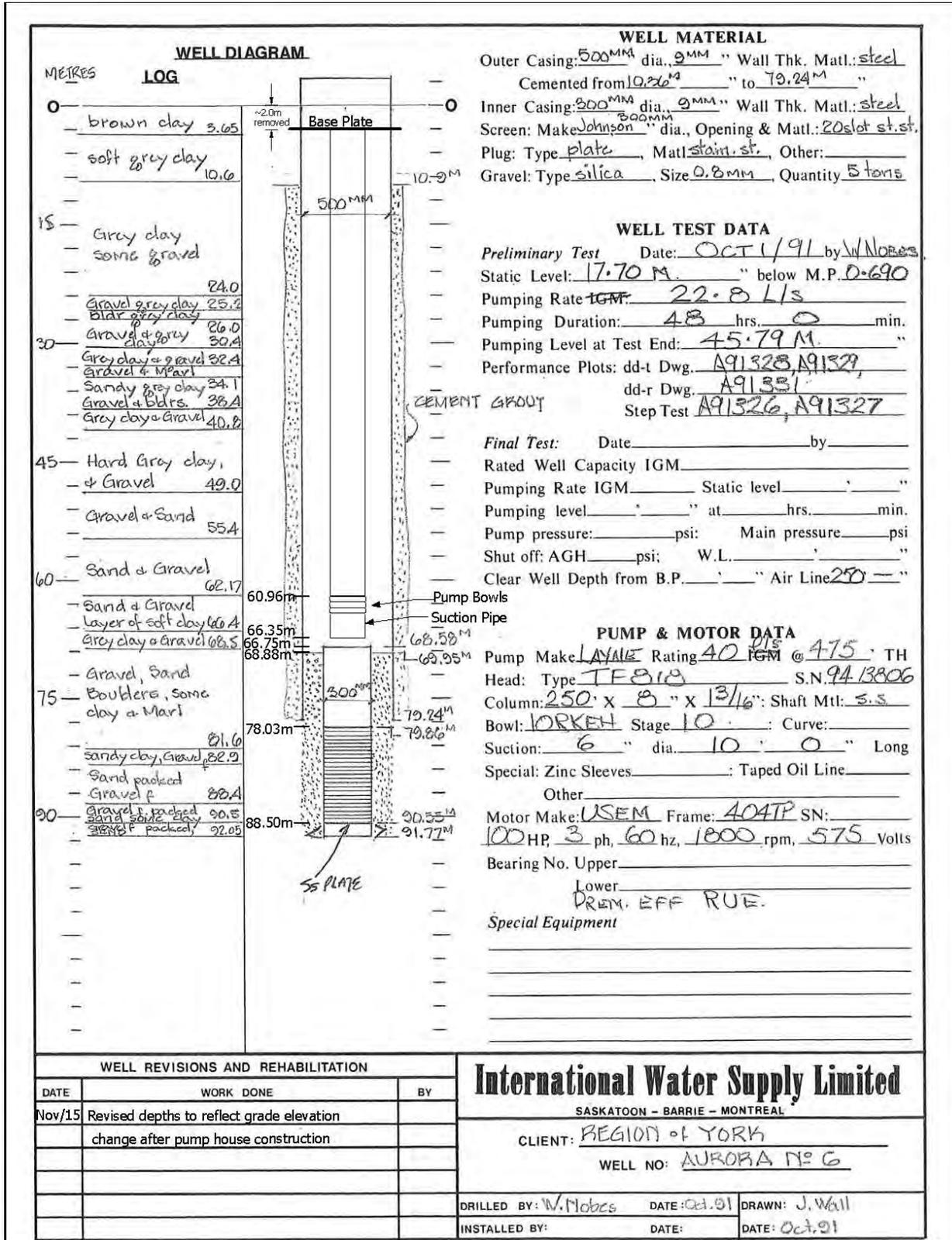
Figure 3. Aurora Well No. 6 Revised Well Diagram (IWS, 2019)
