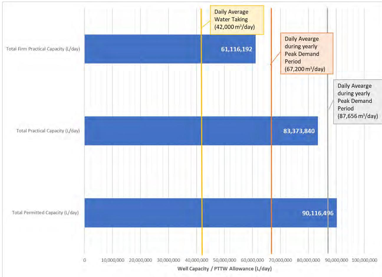
Figure 8. Comparison of YSA Well Capacity and PTTW Daily Limits
