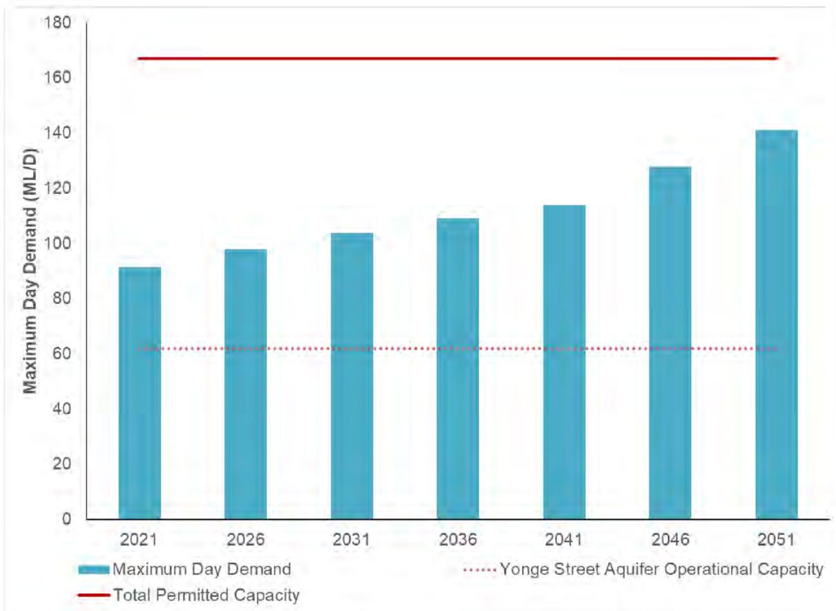
**Figure 1. Forecasted Maximum Day Demand and Supply Capacity in Aurora, East Gwillimbury, and Newmarket (Source: 2022 York Region Water and Wastewater Master Plan)**
