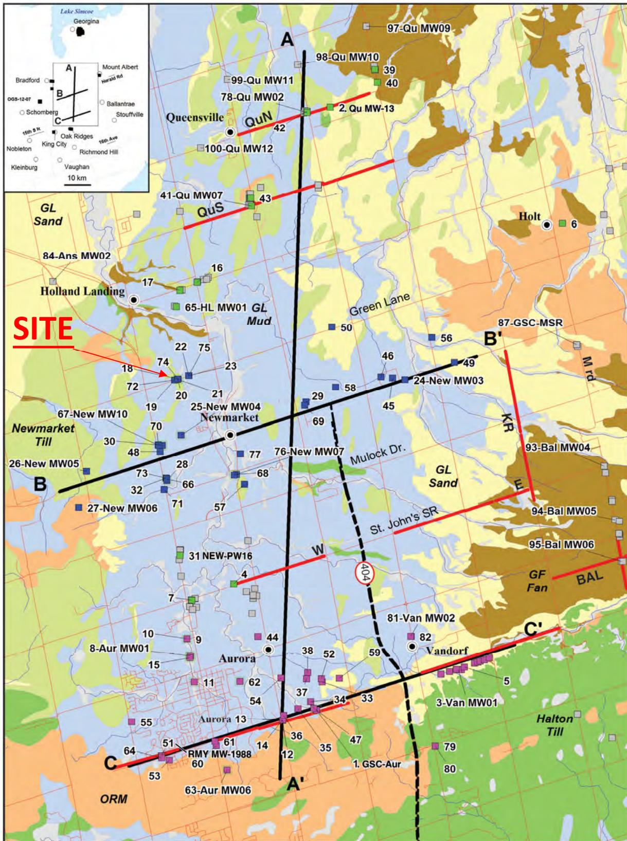
**Figure 6. Geologic Transects across the Yonge Street Aquifer Area (figure adapted from Gerber et al., 2018).**
