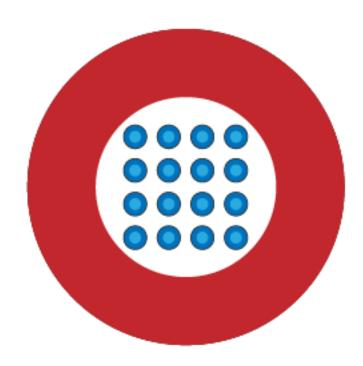
One fibre optic cable can hold hundreds of strands of optical fibre. Typical fibre optic cables hold up to 144 strands.
