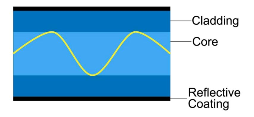
The cladding and reflective coating help light travel through the core without escaping.
