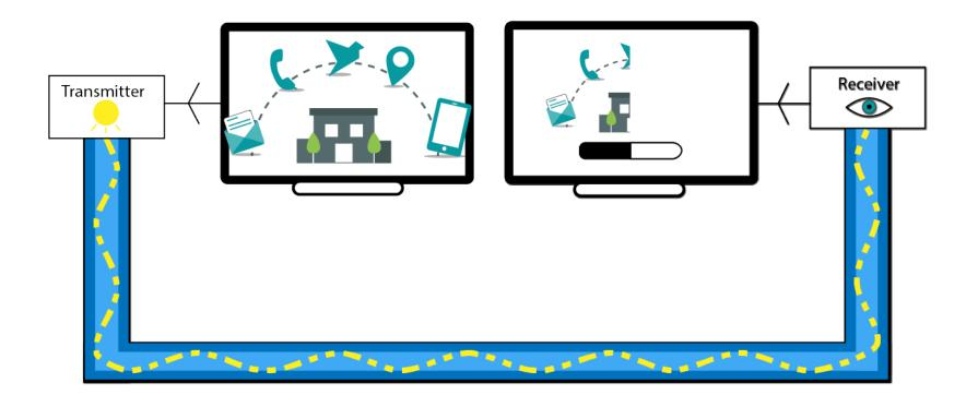
Dark fibre is the 'un-lit' strands of fibre optic cable – similar to an empty pipe.
