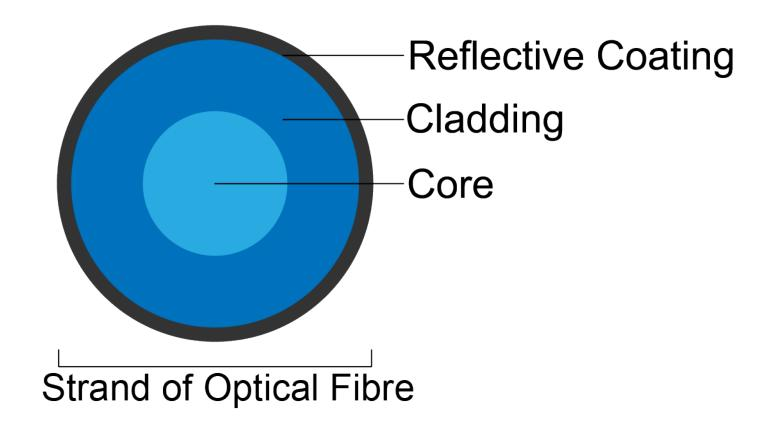
A strand of optical fibre has three layers. The core transmits light, and the cladding and reflective coating prevent light from escaping.
