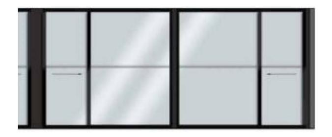
2" Vision strip located at 1350mm above the finished floor provided on all glass panels and doors
