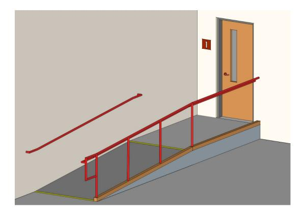
Slope, handrails, landings, and colour contrast strips
