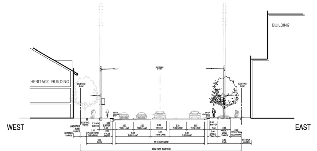
Figure 87: Concept C | Section F-F
