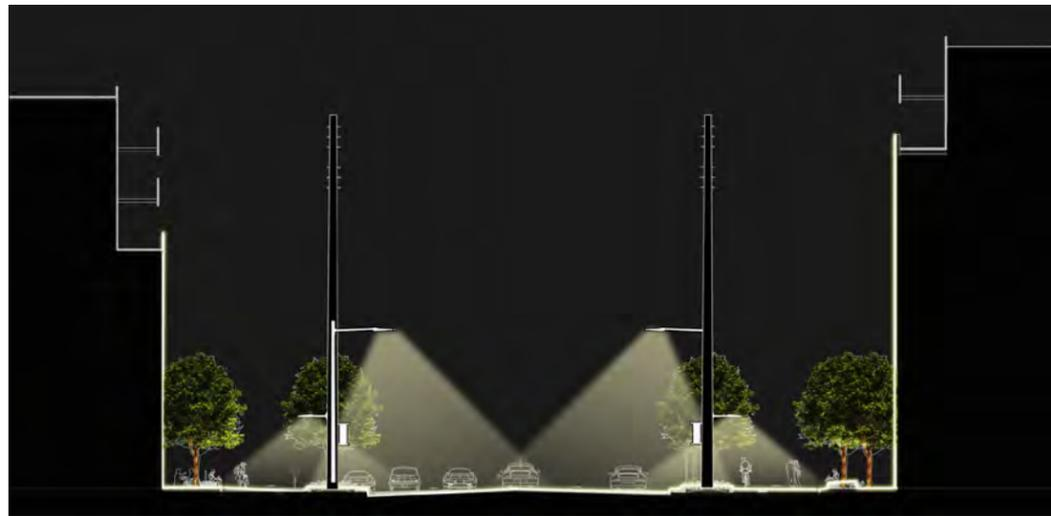
Figure 125: Hydro Poles lights section
