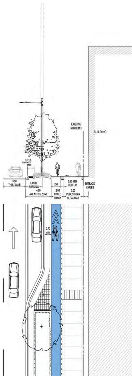
**Figure 55:** Option 1: Cycle Track protected by 2.5m lay-by parking with min. 0.7m “dooring zone” from cycling facilities and by min 0.2m buffer strip adjacent to Pedestrian Clearway.
