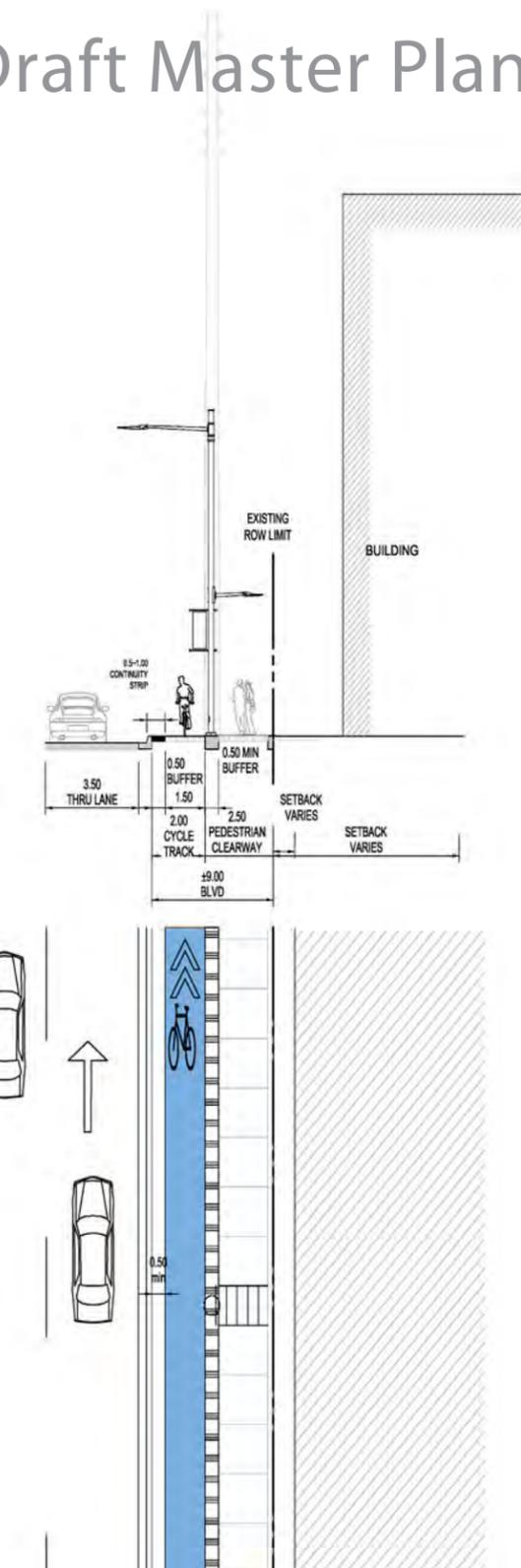
**Figure 57:** Option 3: Cycle Track protected by 0.5m min buffer strip within Continuity Strip adjacent to the roadway and by min 0.5m buffer strip adjacent to Pedestrian Clearway
