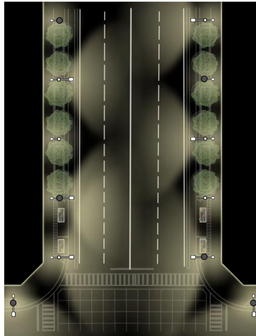
Figure 126: Hydro Poles lights plan view
