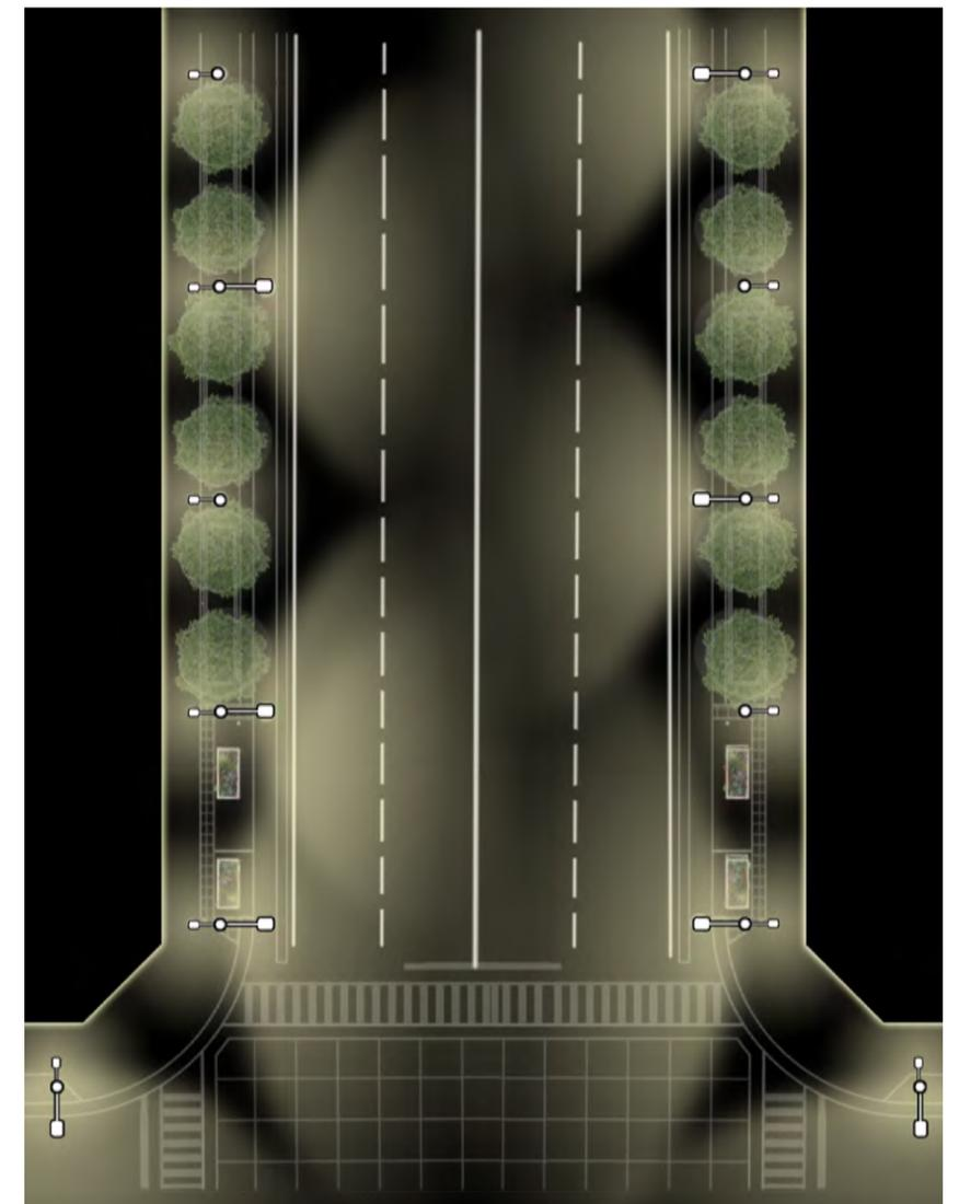
**Figure 124:** Pedestrian and street lights plan view
