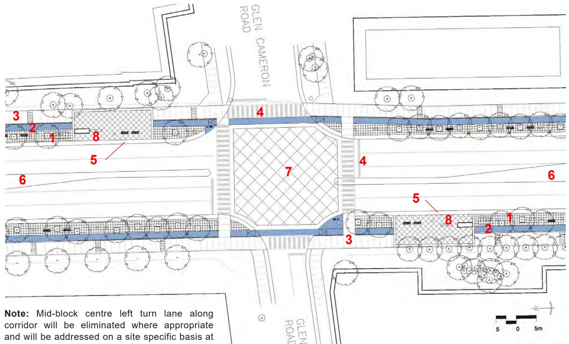
**Note:** Mid-block centre left turn lane along corridor will be eliminated where appropriate and will be addressed on a site specific basis at design development stage.
