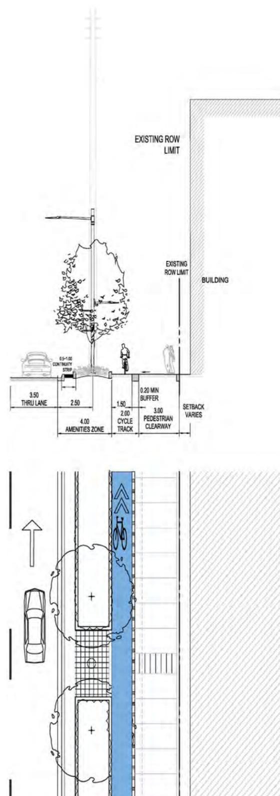
**Figure 56:** Option 2: Cycle Track protected by 4.0m Amenities Zone raised planters and by min 0.2m buffer strip adjacent to Pedestrian Clearway
