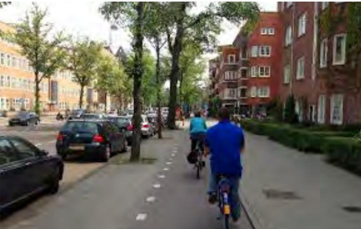
Figure 47: Lay-by Parking is located in-line with the Furnishing and Planting Zone
