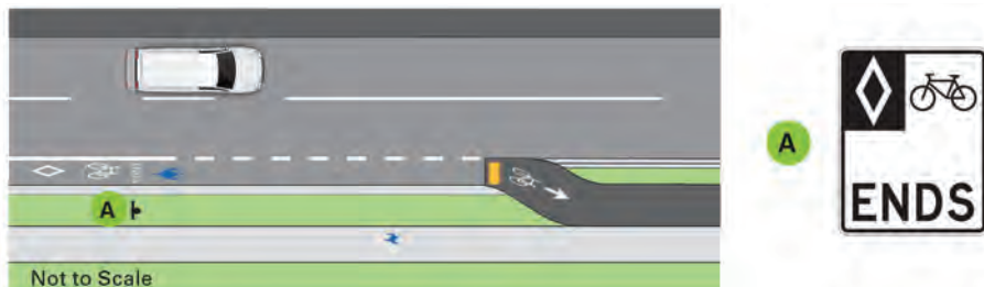
Exhibit 5-11. Bike Lane Ramping up into Boulevard
