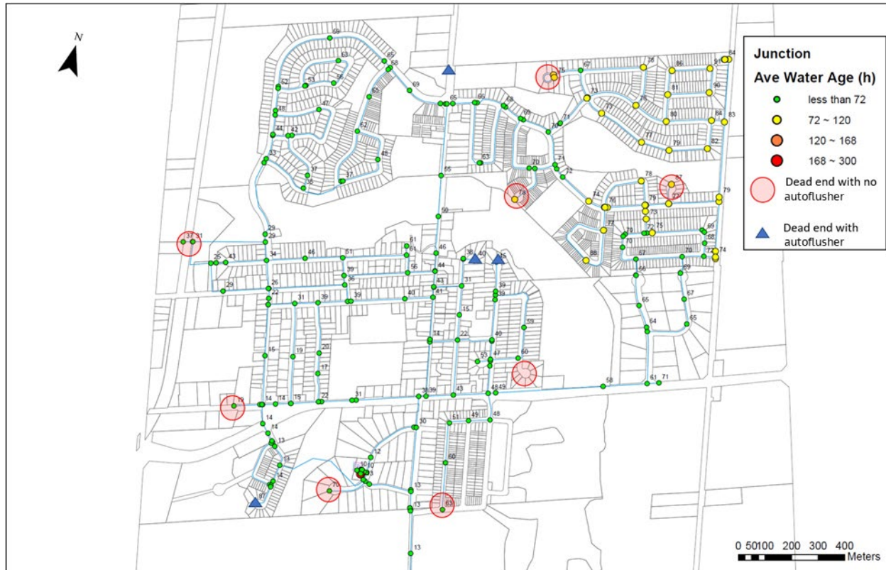
Figure 2-12. Average Water Age (hours) in Mount Albert Water Supply System Showing Location of Dead-Ends and Autoflushers
