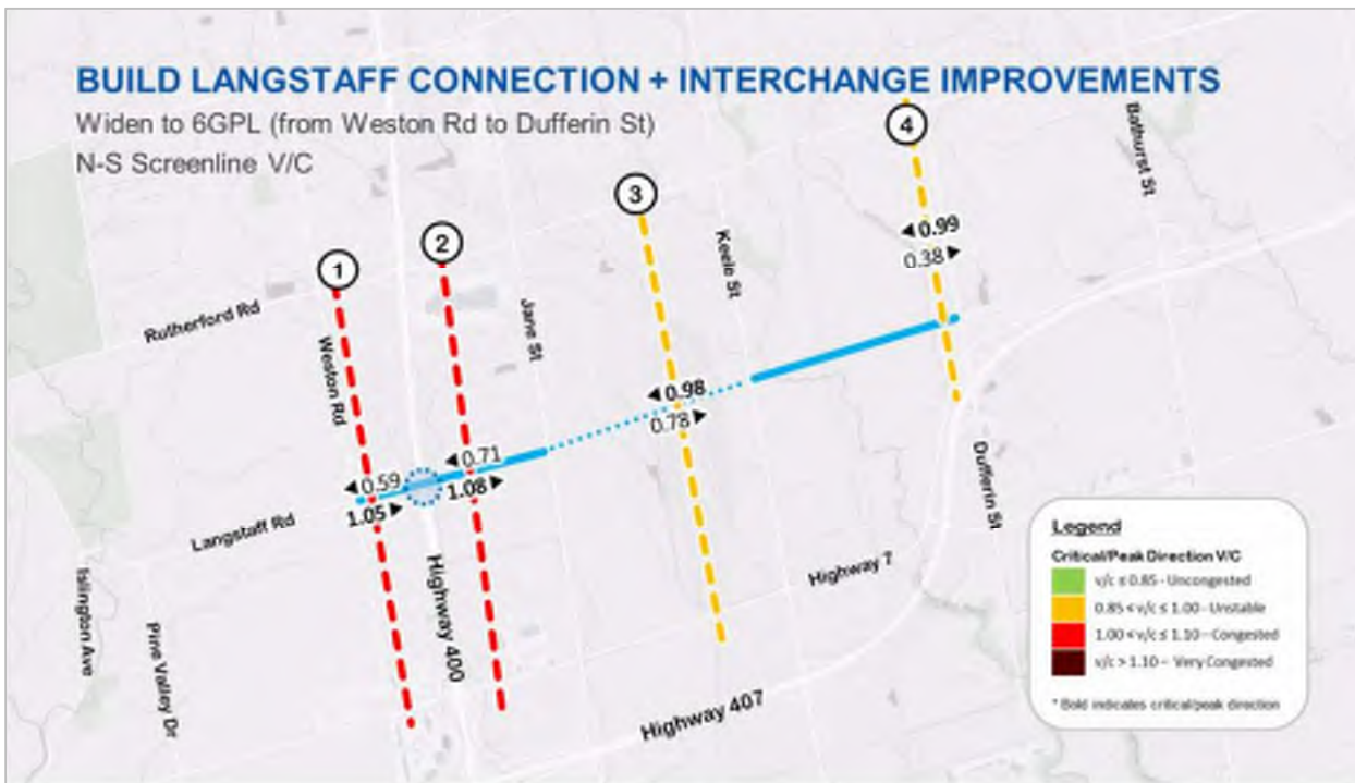
Figure 3-22. Future Build Connection, 6-GPL and Full IC - AM Peak Hour North-South Screenline V/C
