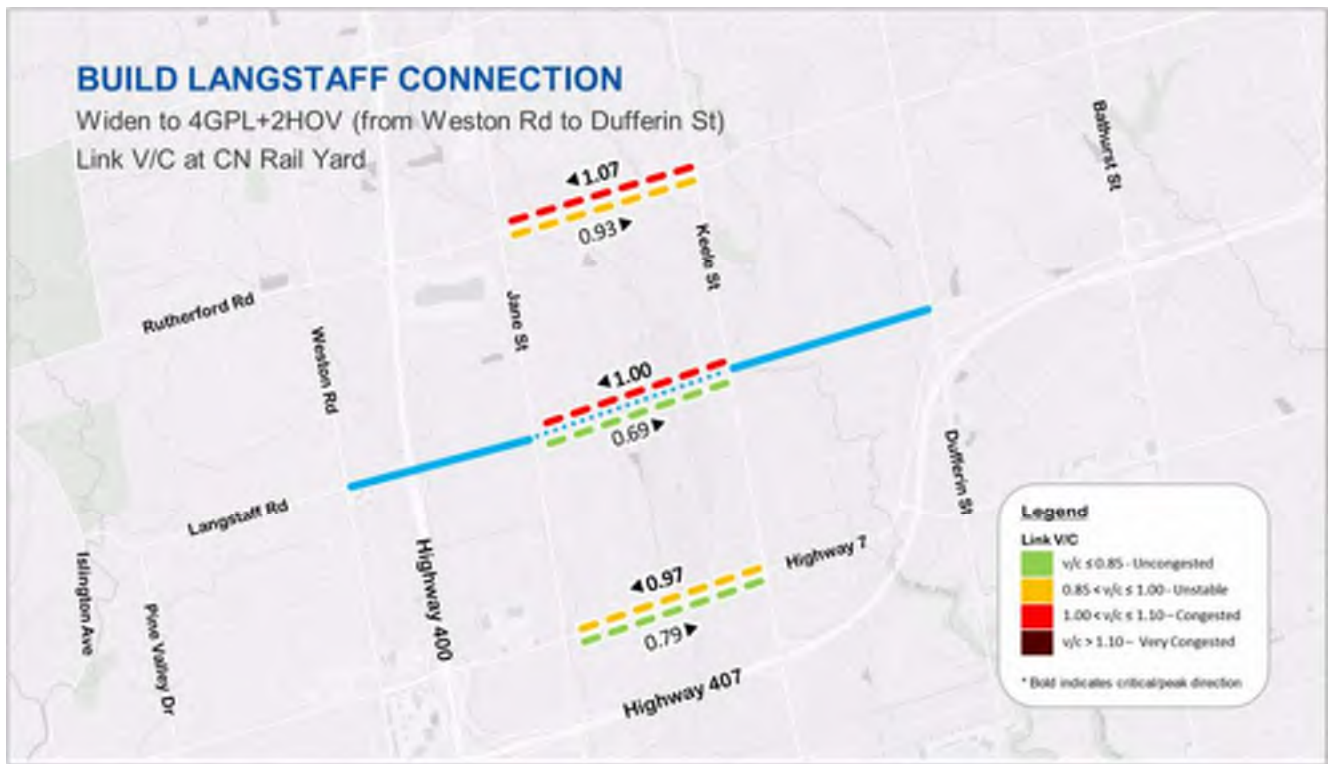
Figure 3-17. Future Build Connection & Transit/HOV Lanes - AM Peak Hour Link V/C at CN Rail Yard
