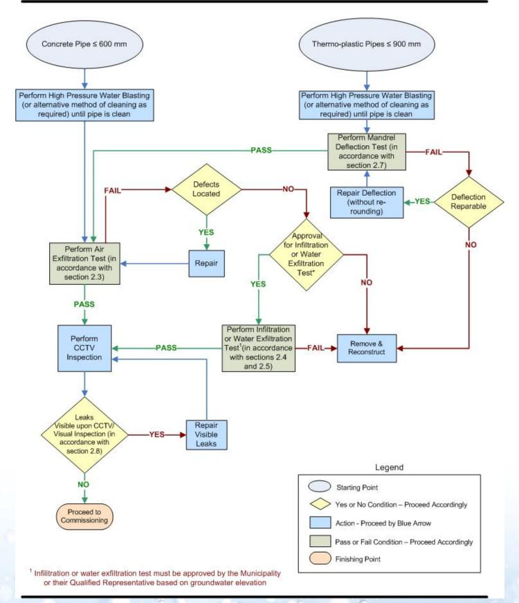
York Region and Local Area Municipalities Sanitary Sewer Inspection, Testing and Acceptance Flow Chart for Concrete Pipes >600mm and Thermo-plastic Pipes >900mm
