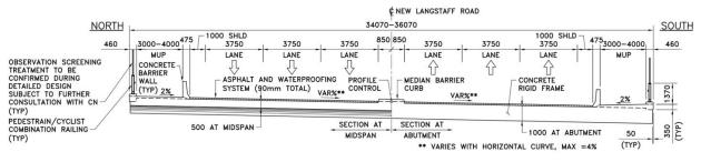
Figure 4: Proposed Cross Section – Approach Rigid Frame
