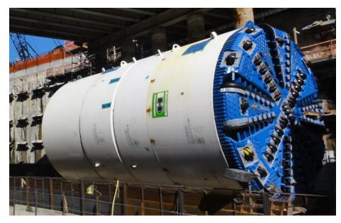
**Pressurized Face Tunnel Boring Machine**
