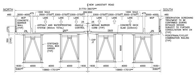
Figure 1: Proposed Cross Section – Main Spans – Steel Box Girder
