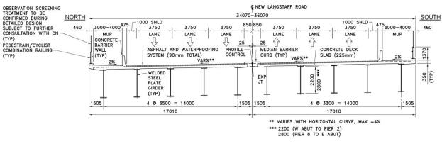
Figure 2: Proposed Cross Section – Approach Spans – Steel I Girder
