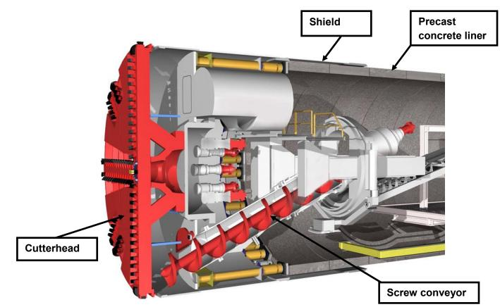
**EPB TBM Schematic**
