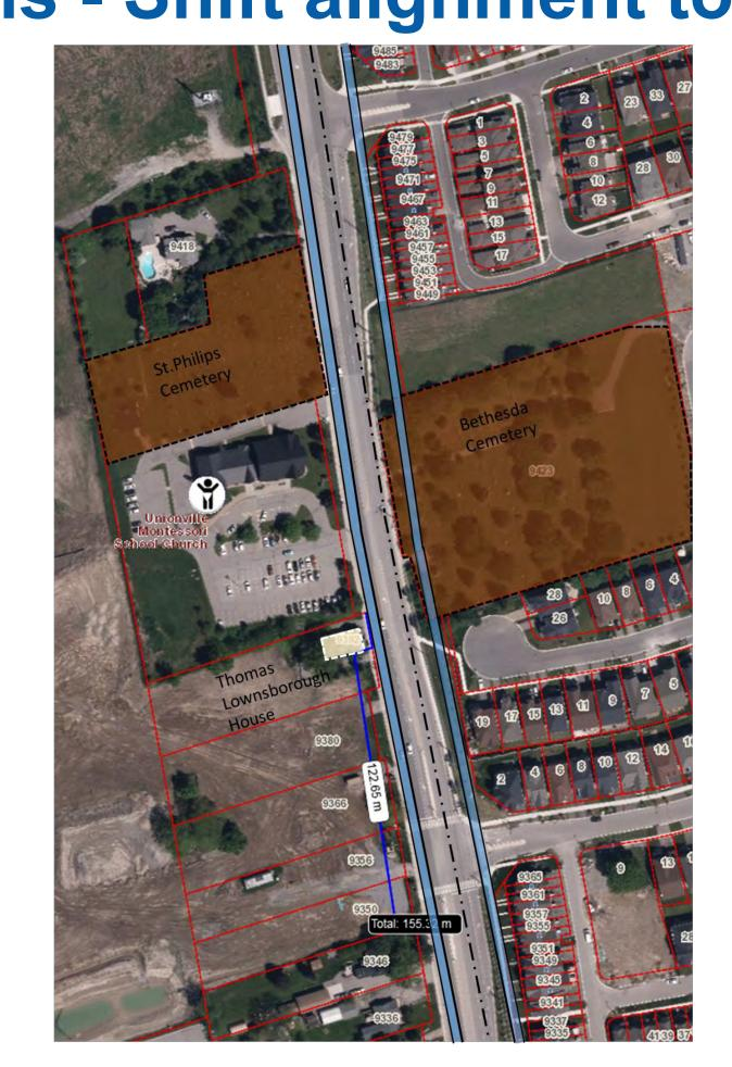
Alternative 4: 6 Lanes with Dual Multi-Use Paths - Shift alignment to the west with discontinuous AT
