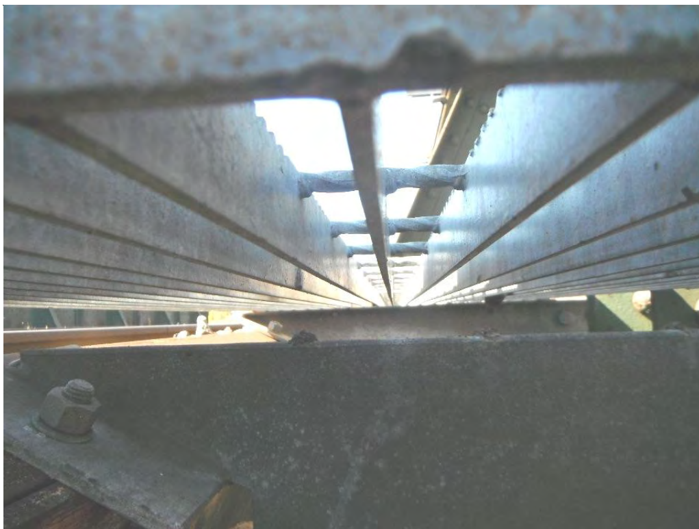
Trainmans Walk not Welded Down
