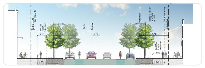
► FIGURE 3: Cross-section of street corridor demonstrating integration of space for multiple modes of travel and utilities. Where feasible, cycling facilities will be relocated to the boulevard.
