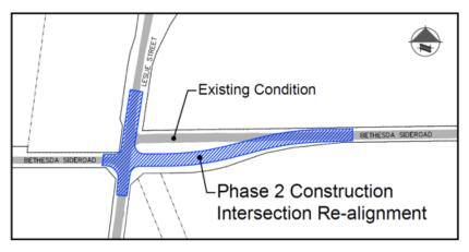
The scope of work includes excavation, grading, ditching, granular material placement, asphalt paving, illumination, road signage and line painting to reconstruct the Bethesda/Leslie intersection and realign Bethesda Sideroad.
