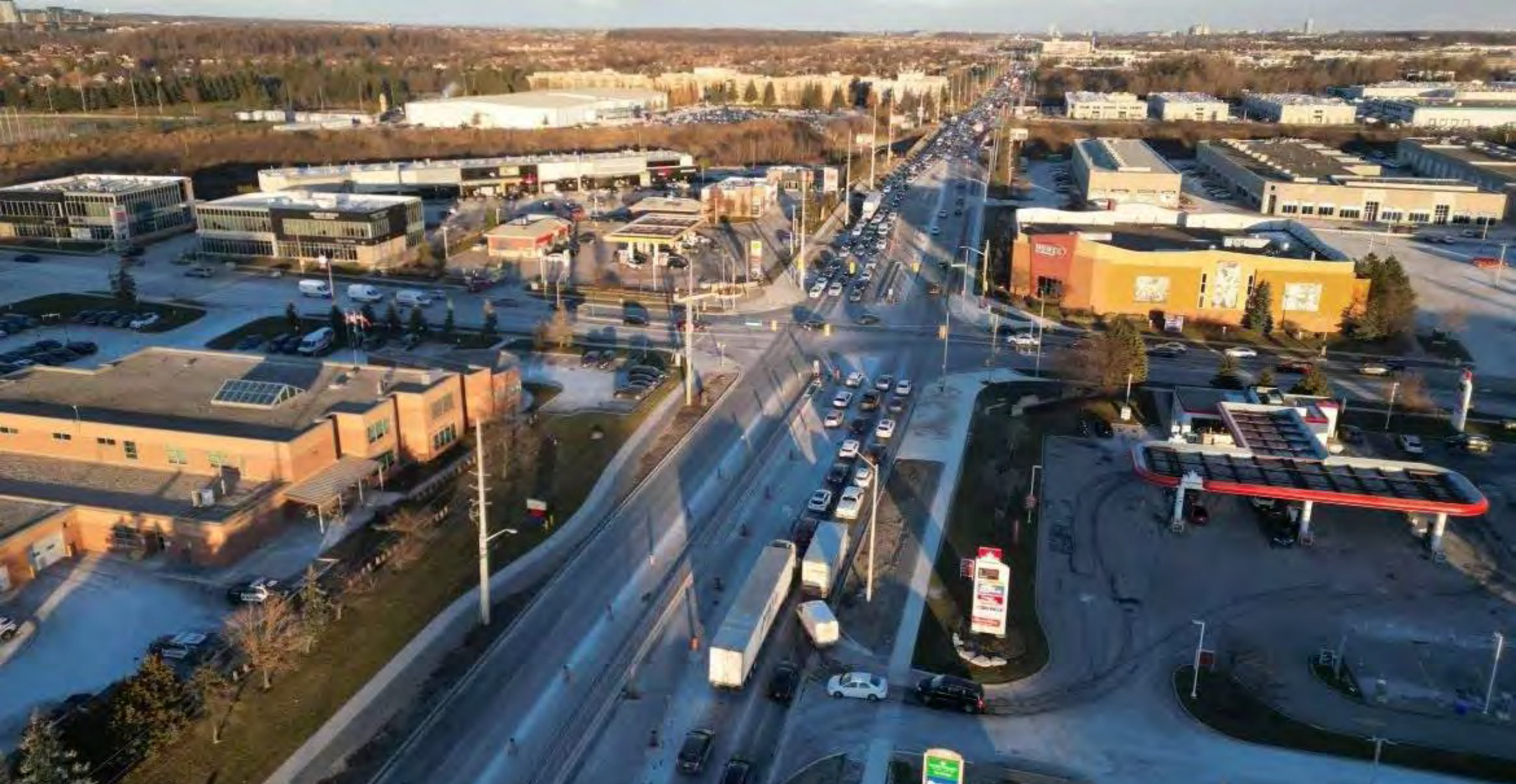
Rutherford Road and Melville Avenue intersection improvements include exclusive left turn lanes to improve traffic flow
