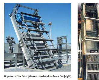
Figure 2-2 Multi-Rake Bar Screens
