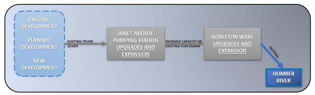
Figure 1-5 Phase 2 Preferred Wastewater Servicing Solution Alternative A: Expand and Upgrade the Existing Janet Avenue Pumping Station and Nobleton WRRF
