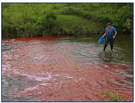
Photograph 7. Humber River immediately following dye injection fully mixed across the river.
