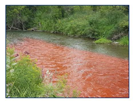
Photograph 8. Humber River approximately 20 seconds after dye injection.
