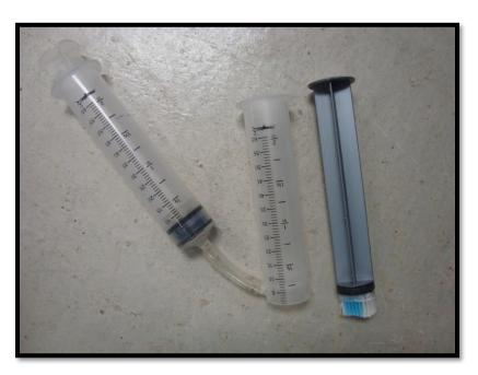
Figure 37. Syringe Sampler for Periphyton Sampling.
