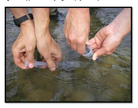
Five replicates were obtained at each location. All subsamples from each site were composited in a 500 mL plastic jar, preserved with Lugol's solution (1/100 mL), kept in coolers or refrigerated until analysis and shipped to ALS in Waterloo, Ontario for taxonomic analysis (species identification and enumeration).
