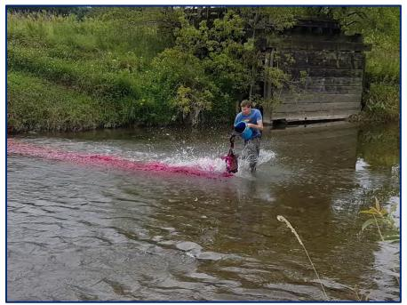
Photograph 6. Instantaneous injection of Rhodamine dye in the Humber River.
