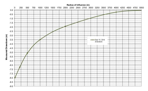
Figure 25. AQTESOLV Forward Solution – Estimated Radius of Influence
