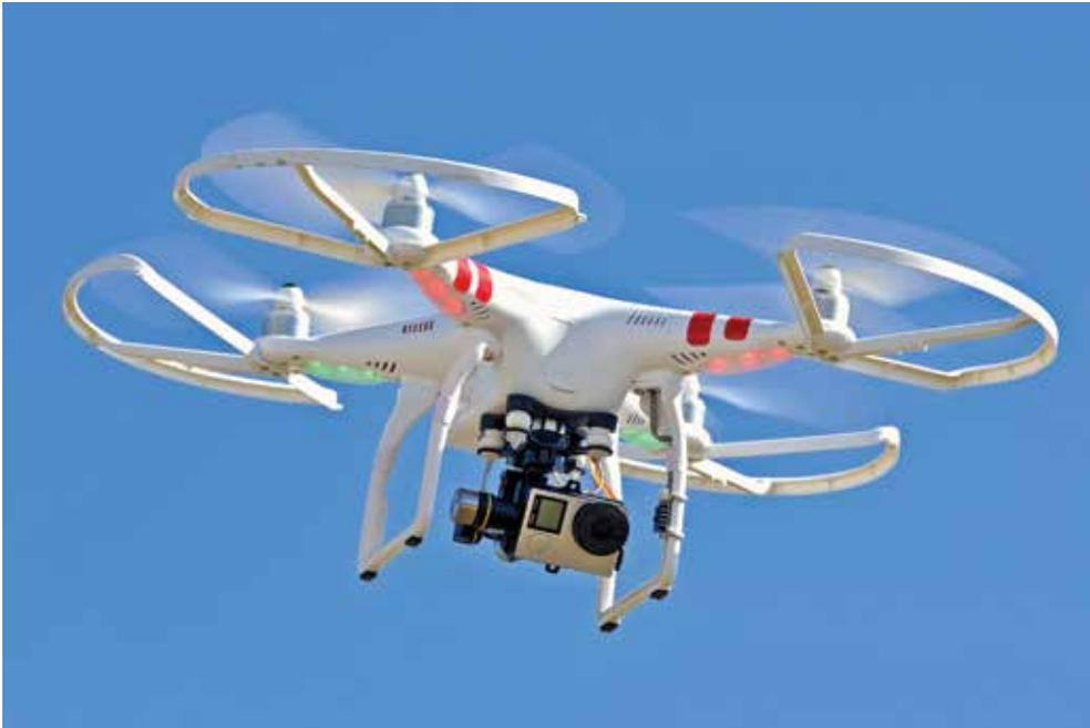
*Drone with mounted camera*
