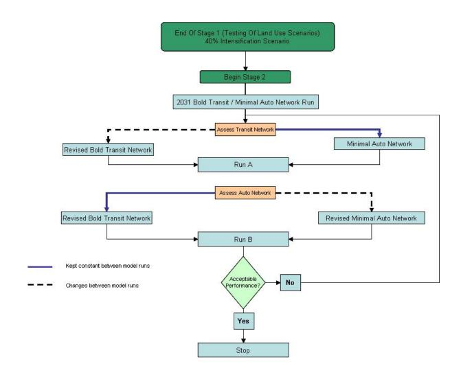
Figure 9. 2031 Recommended Network Development Process
