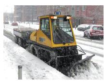
Maintenance vehicles for facilities separated from the roadway: Tractor width: 1.1 to 1.2 m typical
