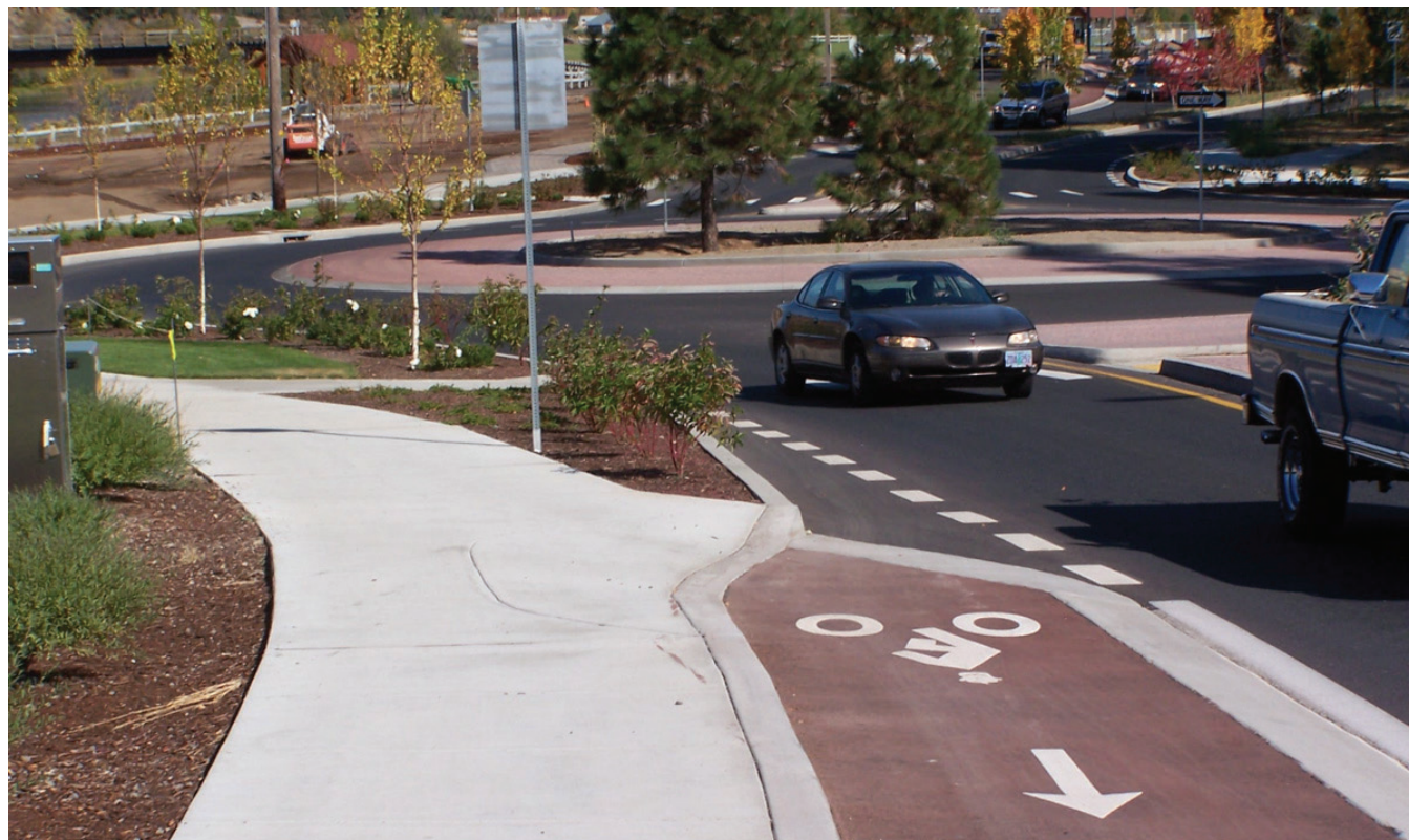
Exhibit 5-63. Example ramp treatment at a roundabout
