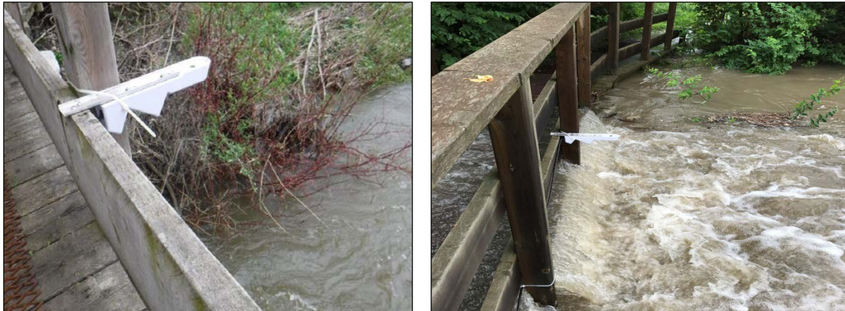
Figure 17 – Down-looking Ultrasonic Level Sensor Monitoring Creek Levels at Aurora Sewage Pumping Station in May (left) and June 23 (right) of 2017
