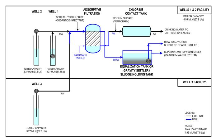
Figure 4-2. Alternative A5a Schematic Diagram
