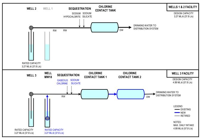
Figure 4-5. Alternative A7a Schematic Diagram
