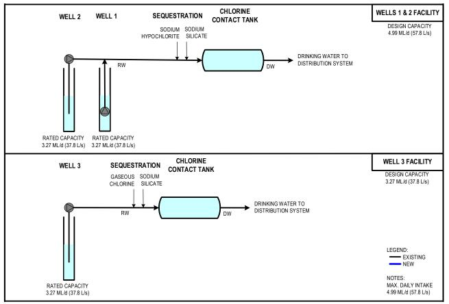
Figure 4-1. Alternative A4 Schematic Diagram
