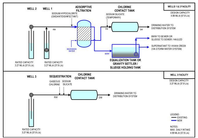
Figure 4-4. Alternative A6 Schematic Diagram
