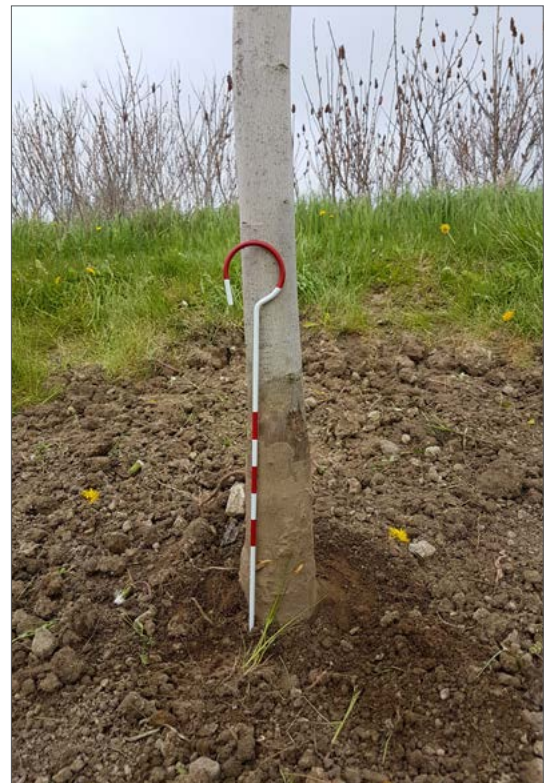
A surveyor's pin can be used by tree planting inspectors to determine excess soil in the root ball of a wire basket tree. Planting depth is one of the most important factors in proper tree planting.
